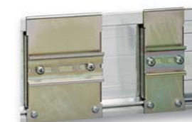
SLZ10 ... SLZ14 Mounting bracket for the S7-300 rail Bracket: Width of unit: SLZ10 up to 40mm SLZ11 41 to 51mm SLZ12 52 to 66mm SLZ13 67 to 90mm SLZ14 91 to 121mm
