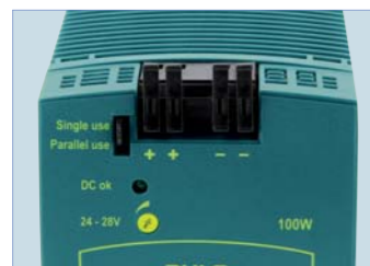
Jumper to select between "single use" and "parallel use". Parallel use enables a current sharing between power supplies.
